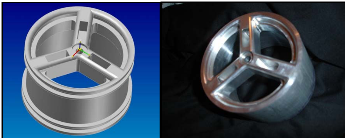
Figure 10. SurfCAM RC Billet Monster Truck Wheel Surface Model & Part
