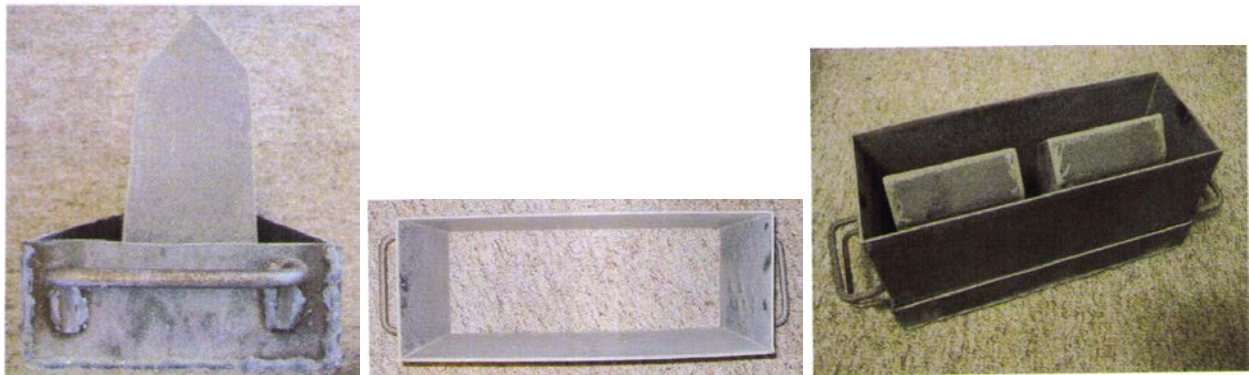
Figure 4: CMU Steel Mold (a) Base, (b) Shell and (c) Assembly
