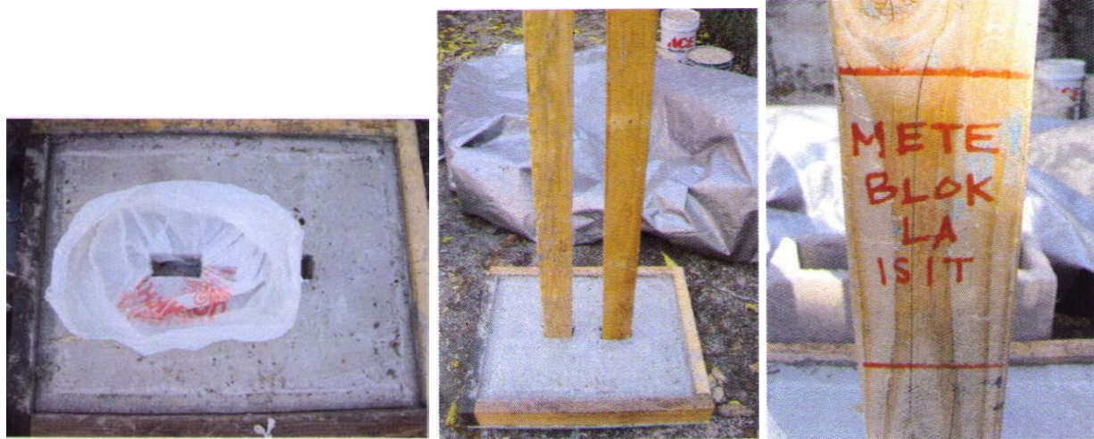
Figure 7: CMU Drop (a) Reinforced Concrete Base (b) Assembly and (c) Positioning Lines after Calibration
