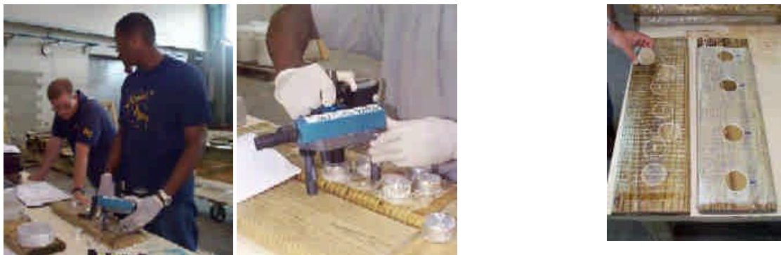
Portable pull-off tester used to measure the bond strength. Samples after adhesion testing Figure 2. RET participants measured the bond strength of their materials before and after various environmental exposures.
