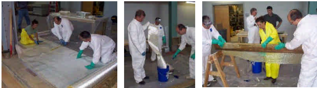
Preparing constituent materials. Impregnating cloth. Fabricating composite-wood beam. Figure 1. RET participants reinforced wooden beams with glass-epoxy composites.
