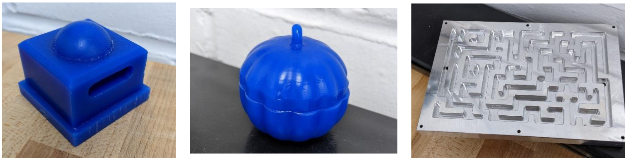
Figure 1: (left) Assignment 1. Stock part manufactured on the 5-axis Pocket NC. (middle) Assignment 2. Student design (candle holder, it opens) manufactured on 5-axis Pocket NC. (right) Assignment 3. Two-sided maze manufactured on the 4-axis Haas VF3.
