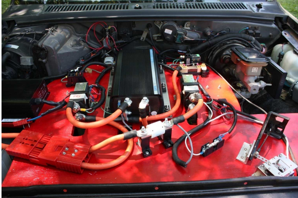
Figure 8: Controller and its circuits
