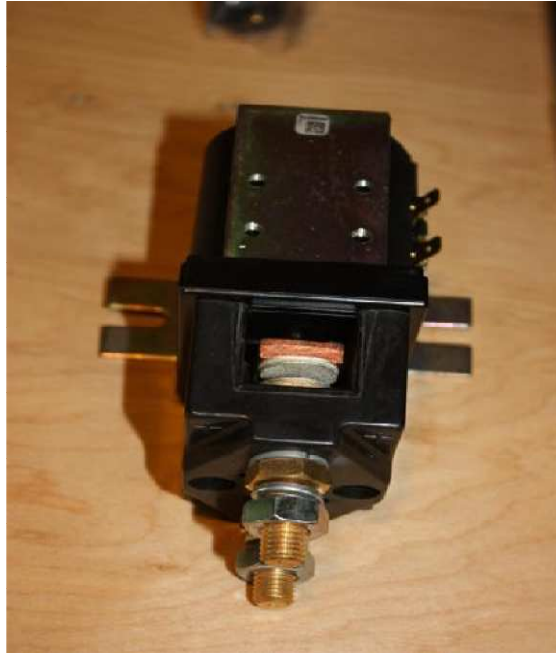
Figure 5: Contactor Used in the Design
