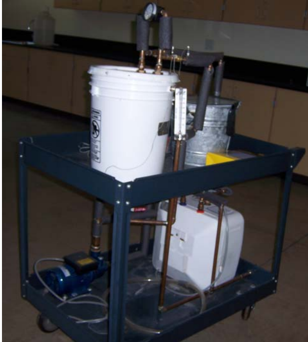
Figure 6: Helical coil heat exchanger experiment.
