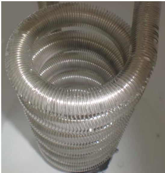
Figure 5: Helical coil used in the heat exchanger experiment.
