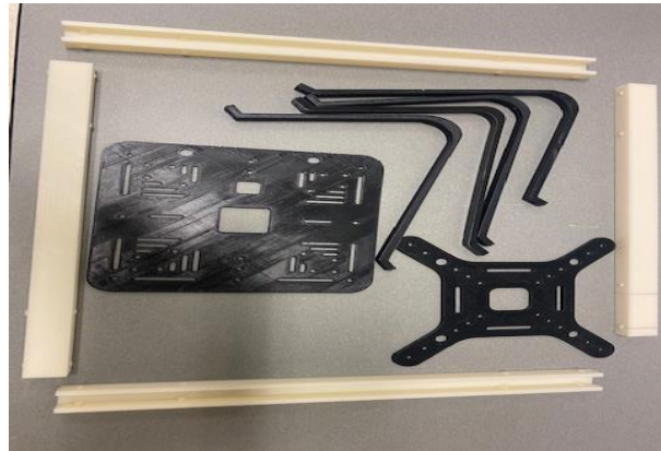
Fig.3: 3D printing of frame components
