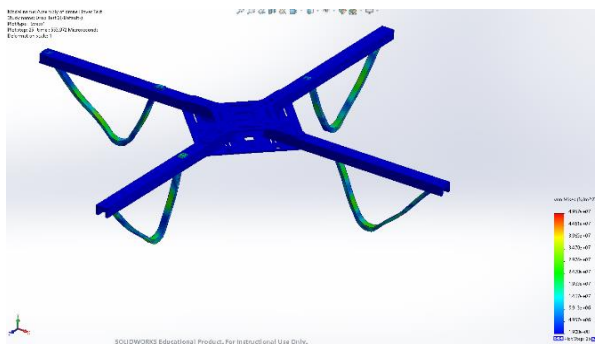
Fig.8: Result of drop test of ELEV-8 drone
