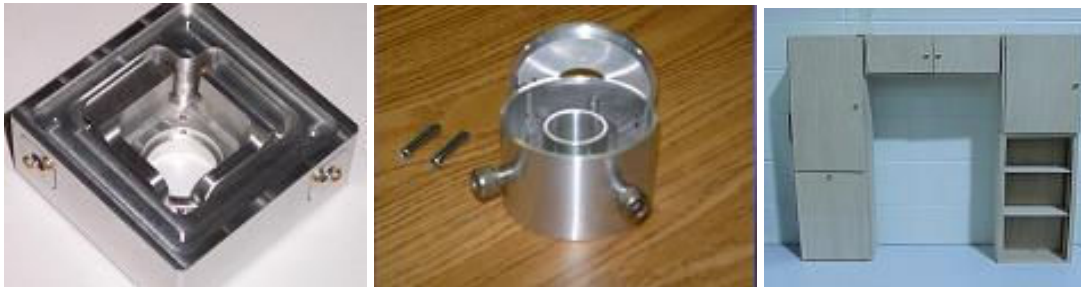
Figure 4. Some representative prototype products developed and fabricated by the students in the capstone design projects, including housing and part of the assembly for a lens directing device (left), the assembly of a low cost laser director (middle), and the wood furniture prototype (right).
