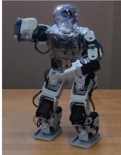
Figure 1. Robotis Premium Type A Humanoid Robot having 18 DOF
