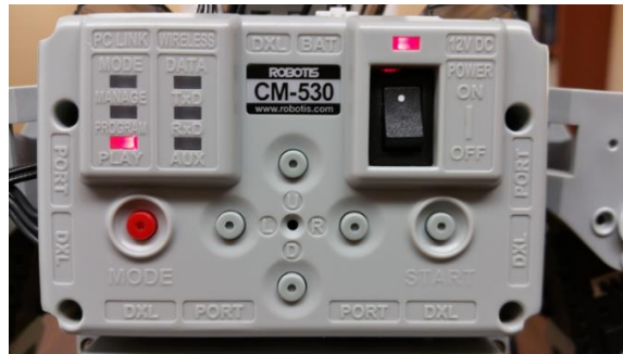
Figure 2. CM-530 Control Module Mounted on the Back of a Robot
