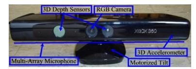
Figure 4. Kinect for Xbox 360 Sensor Package
