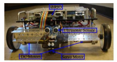
Figure 2. DaNI with Mounted Ultrasonic Sensor
