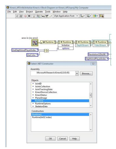
Figure 5. Screen Shot of Initialize Kinect VI Runtime .NET Constructor Change
