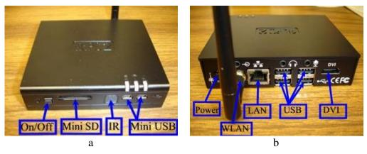
Figure 3. Fit-PC2, front (a) and back (b)
