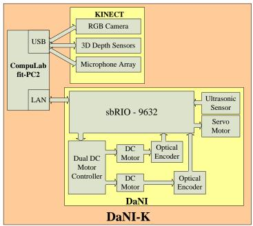
Figure 1. DaNI-K Robot Hardware Block Diagram
