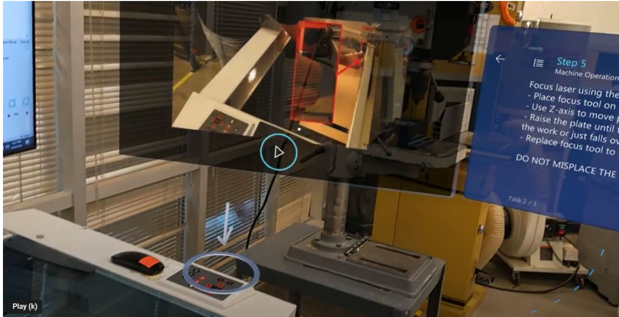
Figure 4 Screenshot from the head mounted device showing superimposed annotations along with a brief video demonstrating the specific steps
