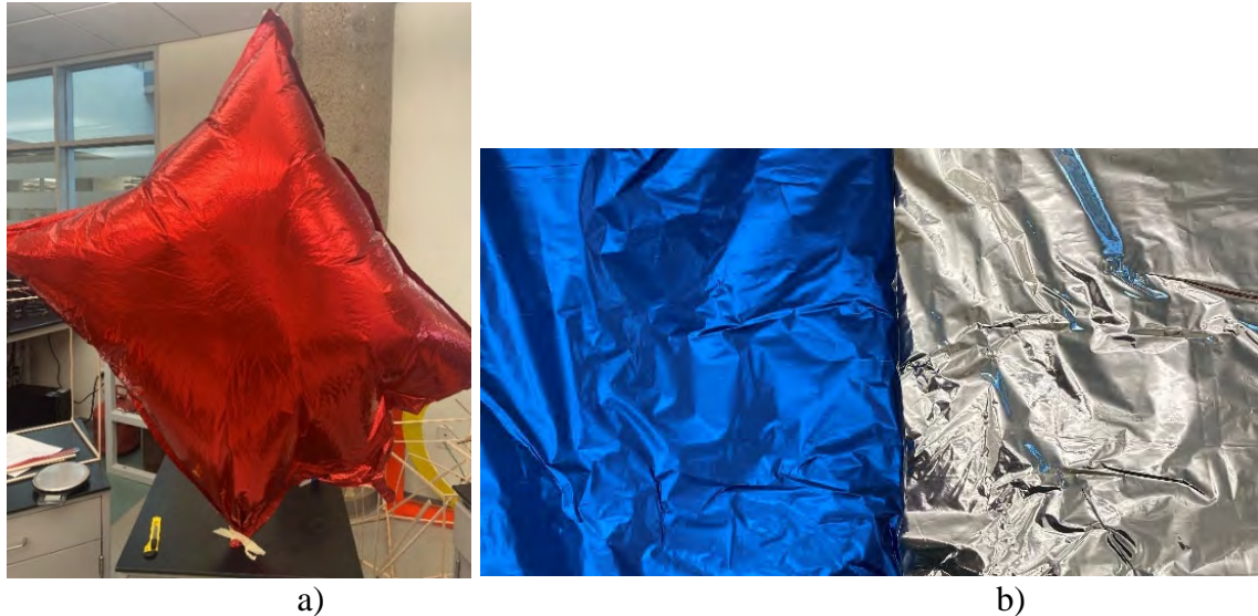
Figure 10. Mylar used for buoyance. a) Image of Custom-Made Mylar Balloons, b) Outside Colored Lining and Inside Silver Lining of Mylar
