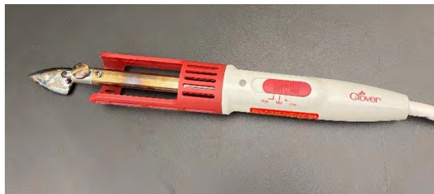
Figure 11: Mini Iron Used for Sealing the Mylar
