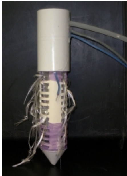
Figure 3. Finished sensor for monitoring moisture content and temperature and obtaining a gas sample.
