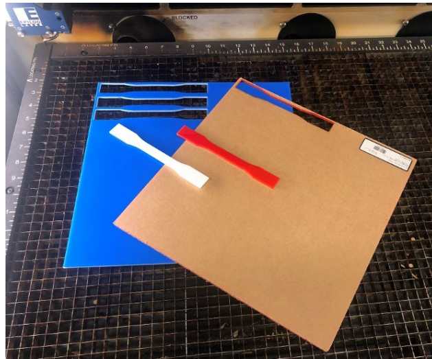
Figure 2 Epilog Fusion M2 laser cutting/engraving machine for tensile sample preparation
