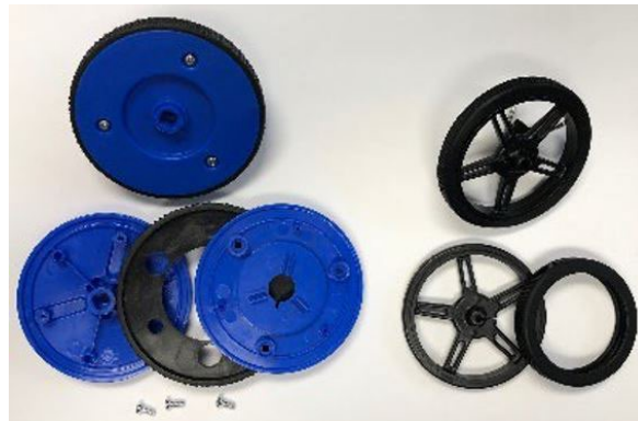
Figure 6 Original MIP wheel (left) and the Pololu 60mm wheel assemblies (right, the rim is not used)
