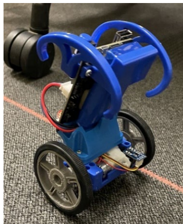
Figure 7 A balancing MIP with redesigned bulkhead and wheel using the Pololu tire
