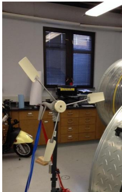
Figure 2. Custom constructed wind turbine blades
