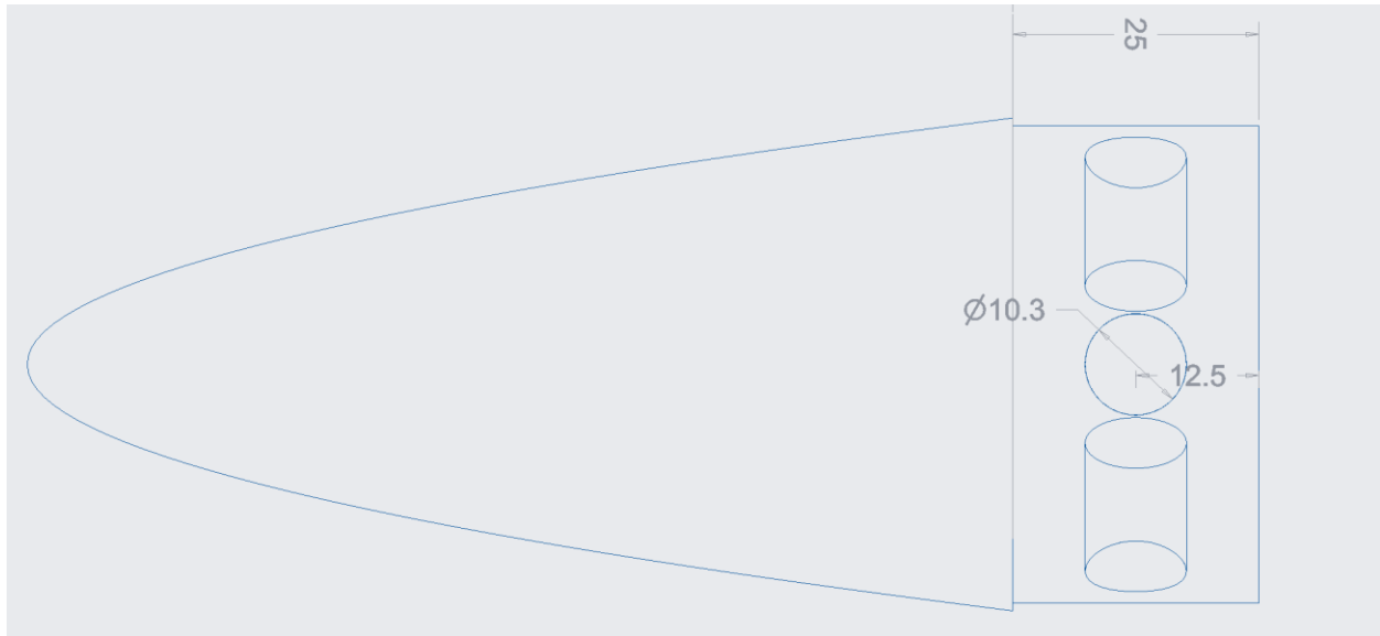
Figure 7. Nose Cone Dimension Design 2
