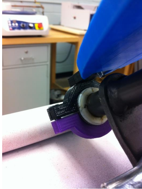
Figure 8: Steering wheel column cover bottom ring connector backside view
