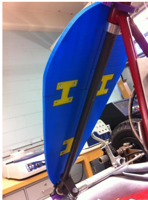
Figure 5: Steering wheel column cover showing connecting pieces backside view
