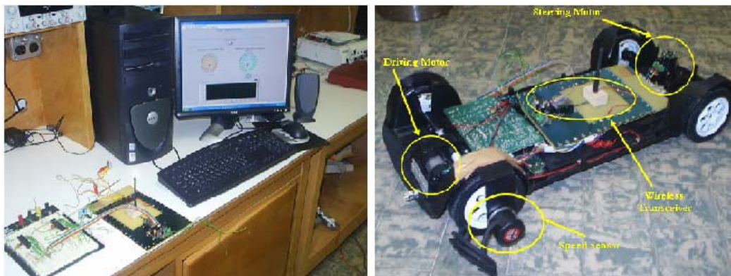
Figure 2 Implementation of the traffic regulation system: (a) base station and (b) model car
