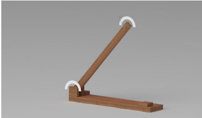
Figure 11. SolidWorks drawing of the hinged bar used in the experiment
