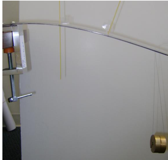
Figure 2. Two-layered beam subjected to tip loading
