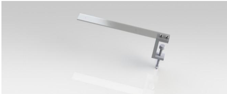
Figure 1. SolidWorks drawing of the unloaded cantilever beam used in the experiment
