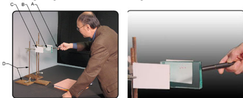
Figure 2 (Left) Experimental set-up: (A) laser pointer; (B) glass plate; (C) screen; (D) stand. (Right) Multiple reflections of a laser beam, shown by the red dots, are captured on a screen.
