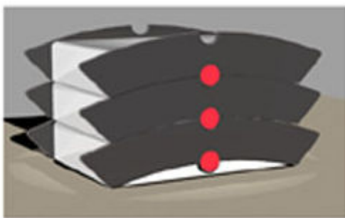
Figure 6. The battery for the laser can be charged by stacking OPTX one on top of another.
