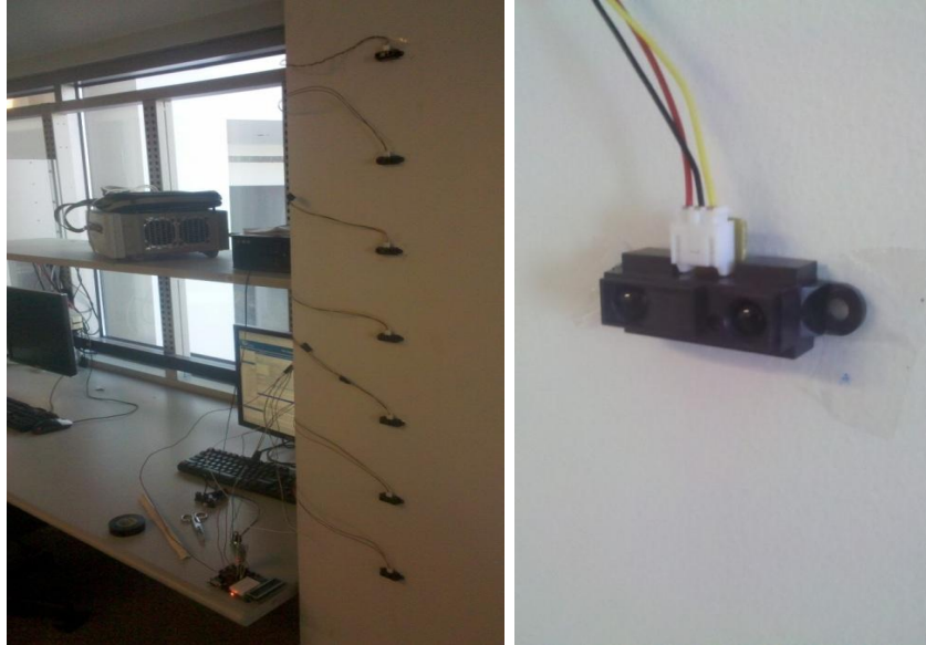
Figure 3(a): Gravity Measurement Project Setup Figure 3(b): IR Digital Sensor
