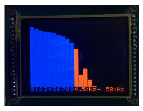
Figure 5: FIR Filter Response Plotted on the TFT Display
