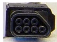
Figure 4. NES Controller Pins with Picture of Connector ( http://www.mit.edu/~tarvizo/nesc-controller.html )
