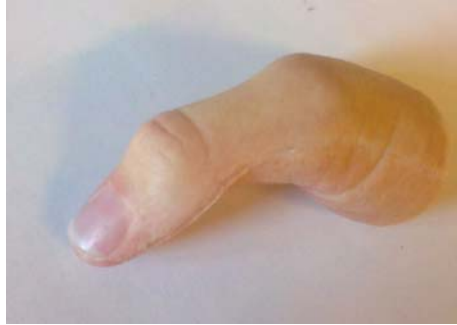
Figure 1: A cast human thumb skin sensor. (Courtesy of Dr. Robert Erb. Made from vacuum-forming 7 layers of silicone foam with detailed painting between coats to match human skin.)
