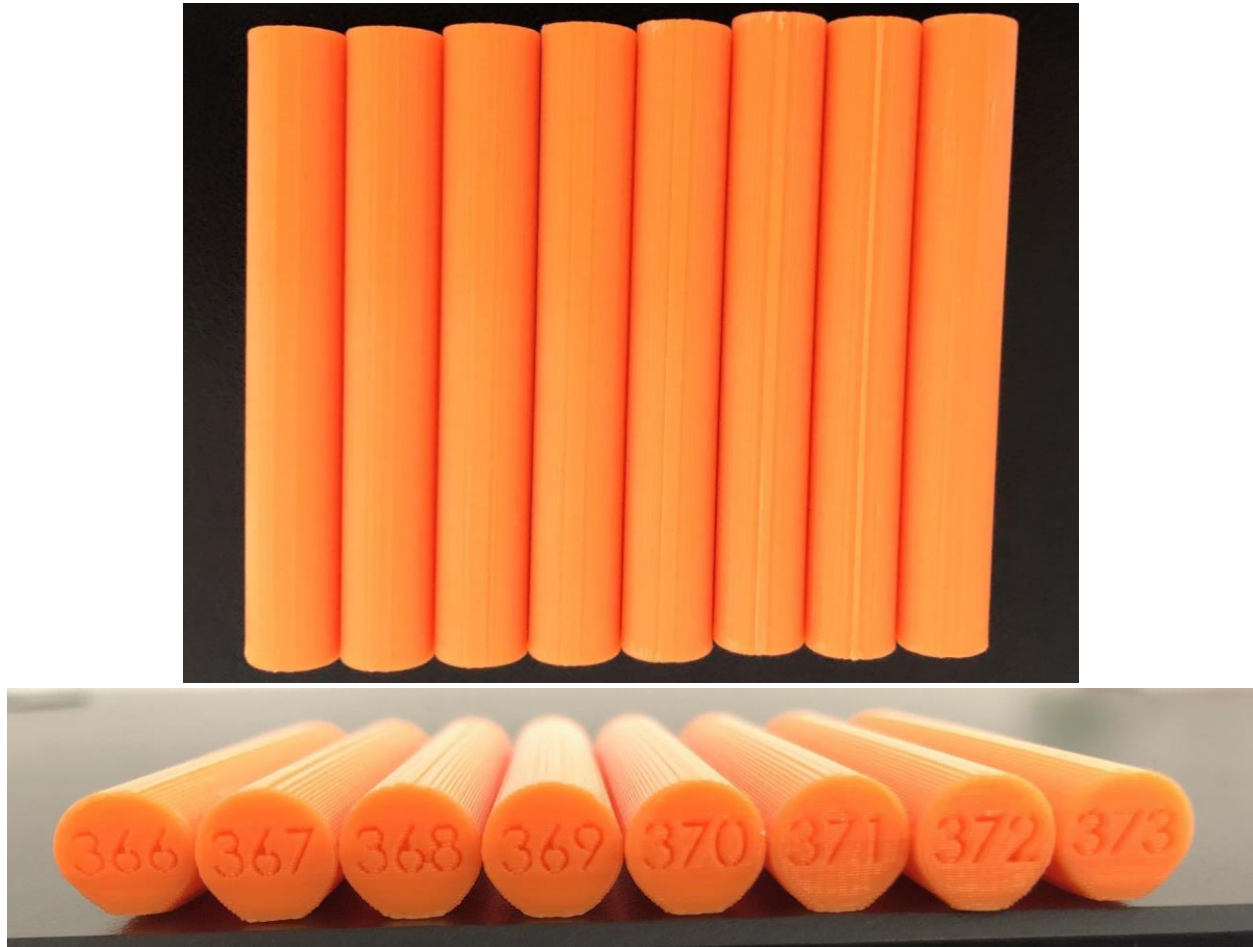
Figure 8: Images of testing shafts used to get the correct diameter used in the final product.
