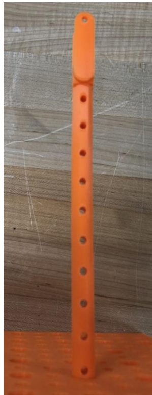
Figure 6: Shows the holes in the pulley shaft to set a certain height.
