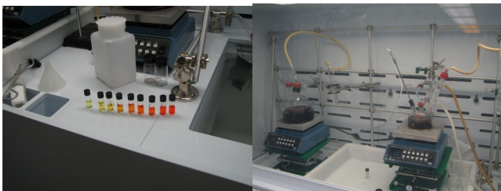
Figure 3 a (left) depicts range of CdSe particles obtained from Junior Nanosystems Engineering students. 2 b (right) are setups of Junior Nanosystems Engineering students for two processes to generate CdSe nanoparticles
