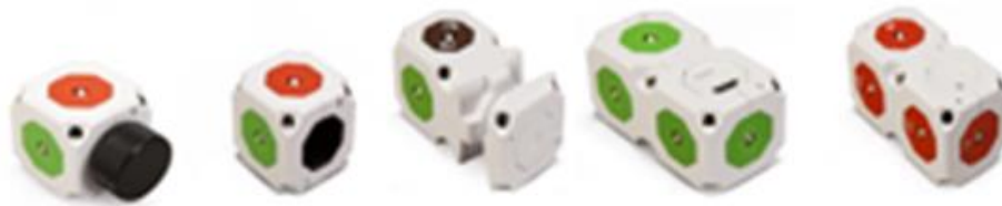
Figure 1. MOSS blocks: knob sensor, mic sensor, motor, power, double-brain blocks. [14][15][16]
