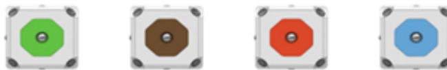
Figure 4. Interface color coding scheme for power (green), data in (brown), data out (red), and pass through (blue) blocks. [14][15][16]
