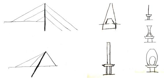
**Figure 5.** Drawings of design alternatives. On the left, drawings of a harp cable arrangement (top) and an inclined tower (bottom). Drawing courtesy of Demi L. Fang. On the right, a series of five single member tower designs. Drawings courtesy of Lu Lu.
