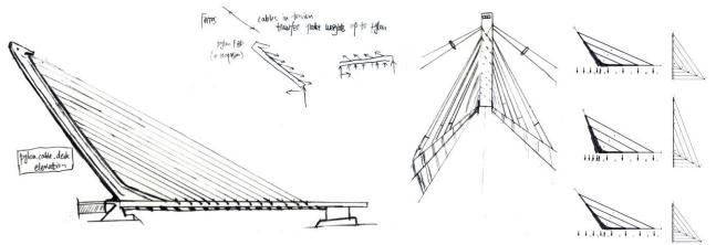
**Figure 7.** On the left and in the center, drawings of Santiago Calatrava's Alamillio Bridge. Inset, free body diagrams. On the right, schematics from eQUILIBRIUM demonstrating the influence of tower angle on the forces in a bridge with no back stays. Drawings courtesy of Lu Lu.
