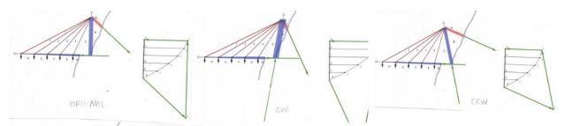
**Figure 6.** Schematics from eQUILIBRIUM demonstrating how inclining the tower in different directions influenced the flow of forces through the structure. Figures courtesy of Michelle Chang.
