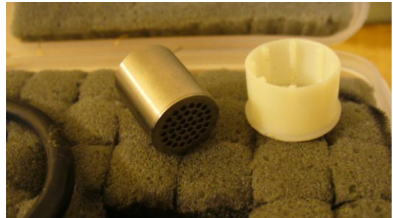
Fig. 6. GenRad 1962, 1/2-inch microphone.
