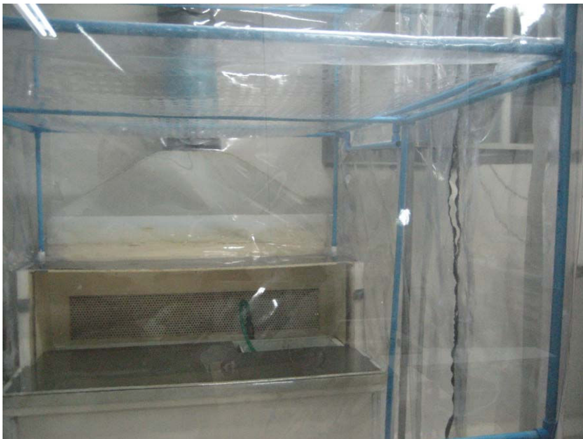
Fig. 2. The wet-etch station as seen through the transparent PVC walls of the cleanroom. The zipper entryway is visible on the right side of the photograph.
