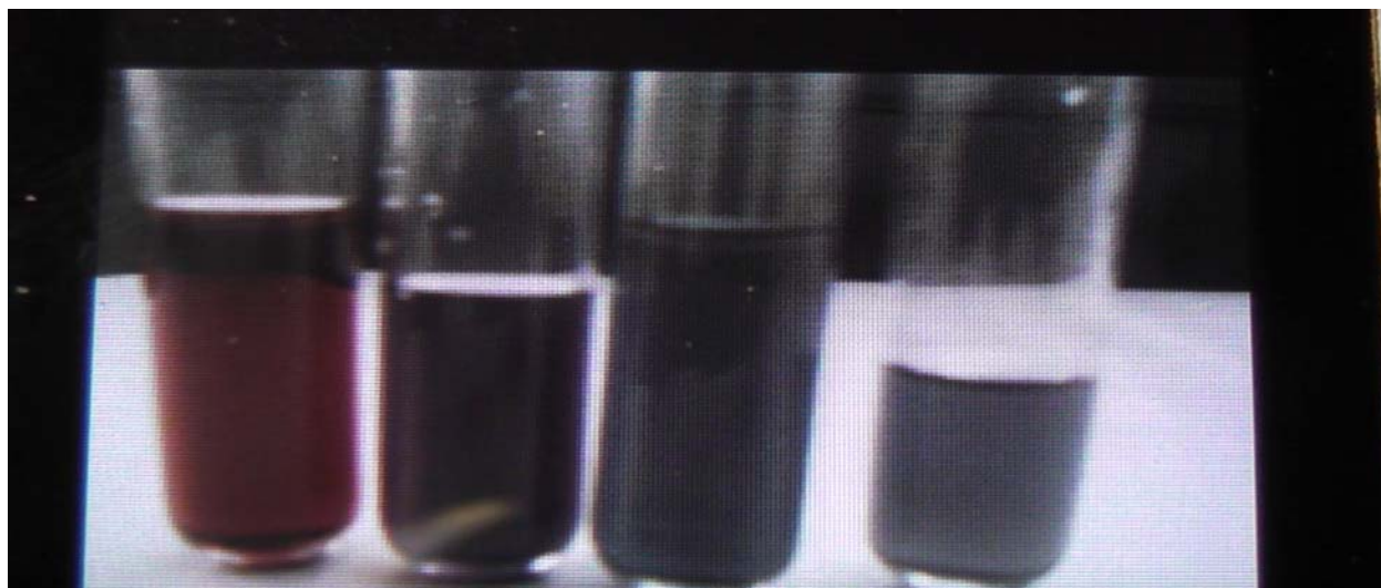
Figure 1 Gold nanoparticles synthesis and the different colors they reflect depending on the concentration of electrolyte in the mixture.
