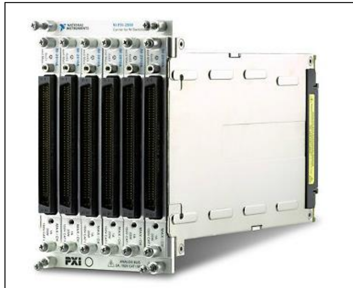
Figure II.2 PXI-2800 - all six of the card slots filled with matrix relay cards.
