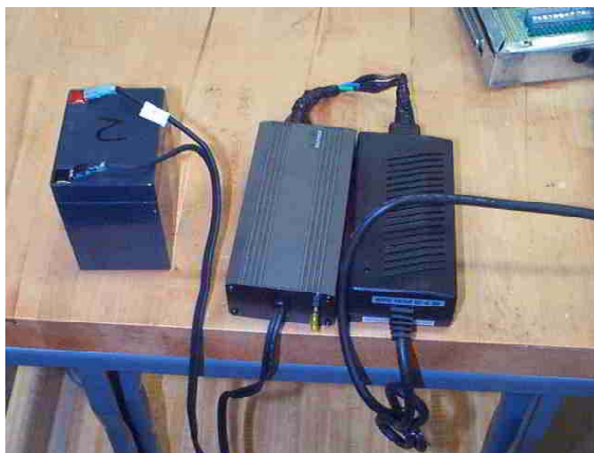
Figure 12: Power system to supply accelerometer signal conditioner
