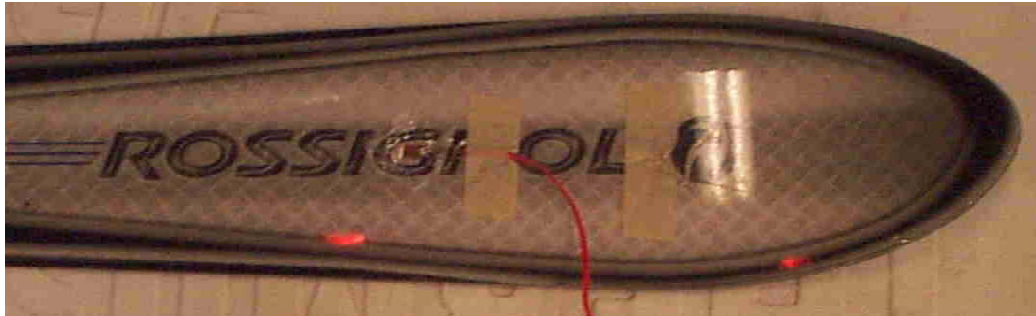
Figure 4: Portion of test ski with single-axis strain gauge
