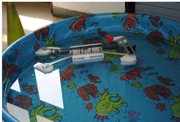
Figure 7. Air propulsion in a floating device
