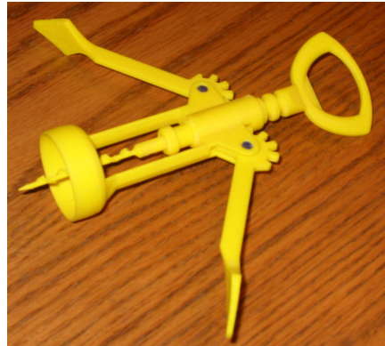
Figure 11 - 3D print of corkscrew design
