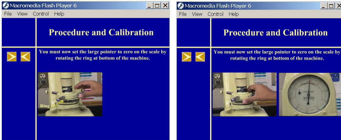
Figure 5. (a) Initializing analog pointer (b) Effect of initialization on the pointer
