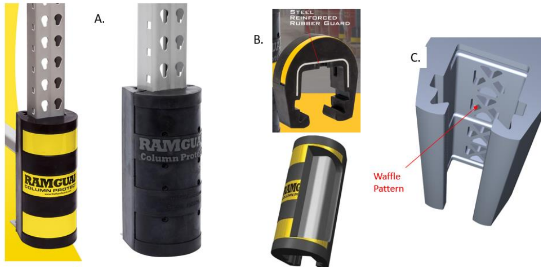
Figure 7: Final column guard design. A. Injection-molded RamGUARD, B. Steel reinforcement column is over-molded into the rubber to increase column strength, C. A waffle pattern is molded into the inside surface to redistribute impact forces to corner of column.
