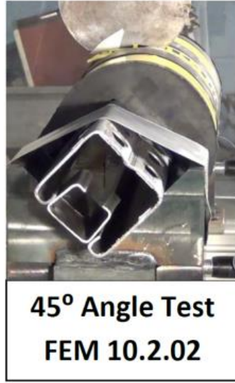
Unprotected 11 gage column after 6 frontal impacts.
