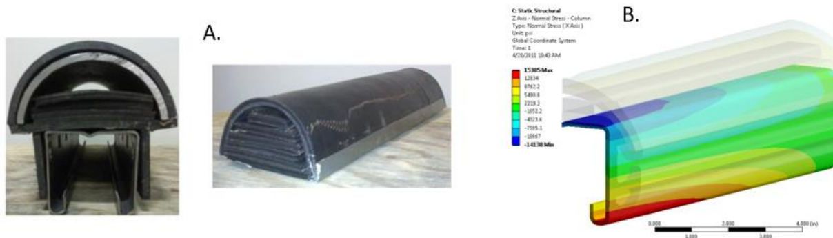
Figure 5: A. Fabricated prototype guards for evaluation, B. Impact simulations performed in ANSYS to validate testing.
