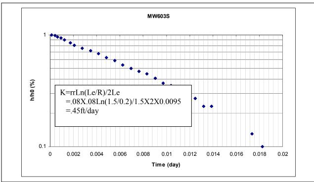
Figure 2, Data, h/h<sub>o</sub>,Vs. time graph and Hvorslev calculation for K, (Hoffner<sup>5</sup>)
