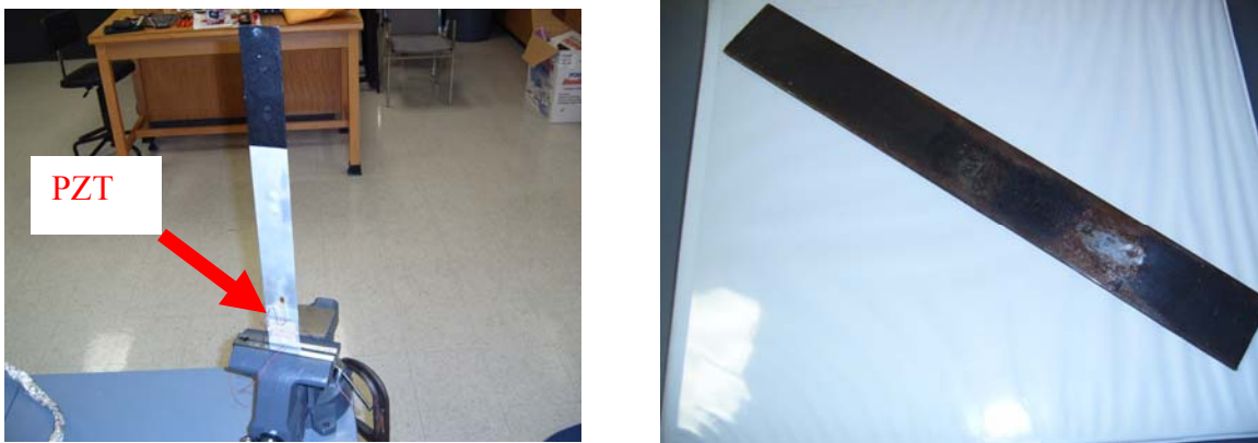
Figure 4: Thin aluminum beam, with mounted PZT (left), and small steel beam (right).
