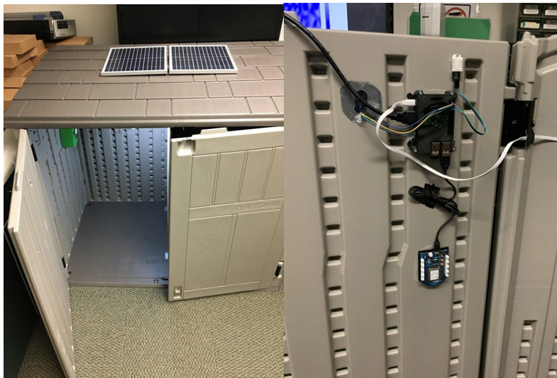
Figure 9: Smart Home Prototype and Coordinator Node [17]
