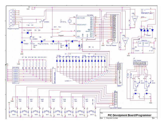
Figure 1. PIC 16F88 Design and Development Platform
