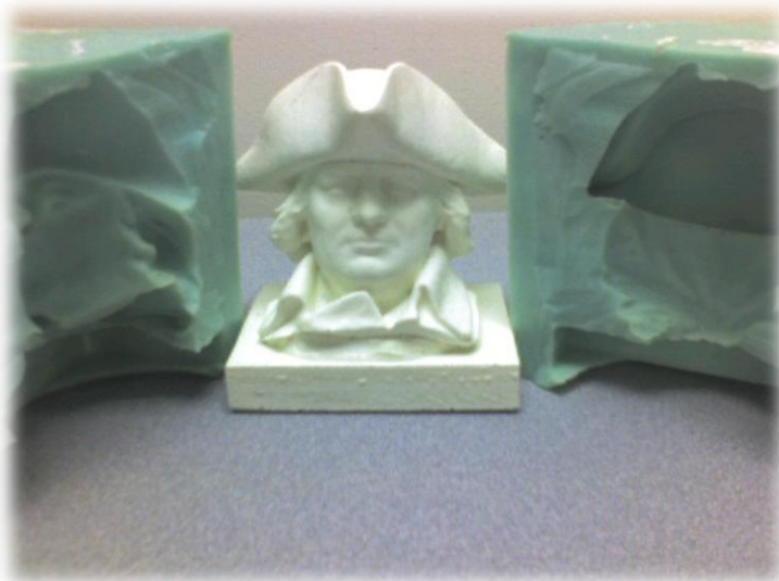
Figure 5. RTV mold halves and resulting polyurethane part
