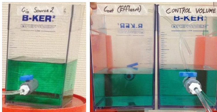
Figure 3. Visual representation of the concentrations with (left) Beaker B exhibiting heterogenous concentration conditions where the completely mixed assumption does not apply and (right) Beakers C and D exhibiting similar concentrations enabled more applicability of the completely mixed assumption.
