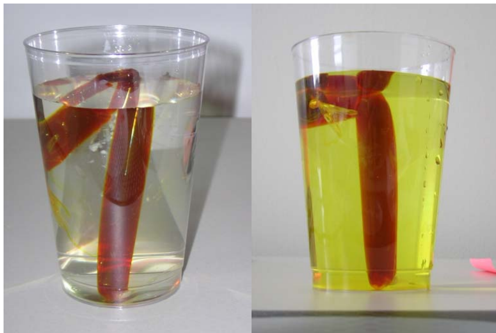
Figure 5: Hands-on activity demonstrating selective diffusion. In this activity students observe the diffusion of a yellow dye out of artificial “blood”.
