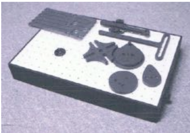
Figure 1, Kinematics kit (stepper motor is inside the box).
