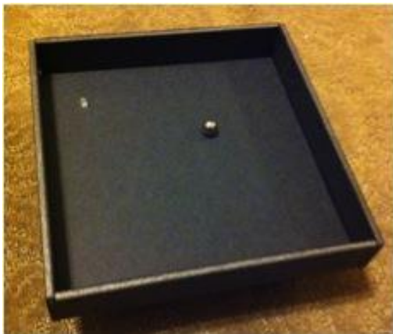
Figure 4a: Top view of the pinball box, showing an LED in the upper left corner and a conductive ball.
