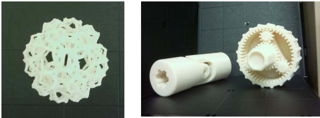
Figure 6 Parts built by a Fused Deposition Modeling rapid prototyping machine 10
