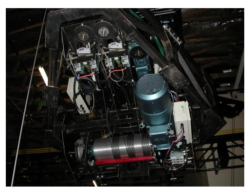
Figure 1. A modern lifting/traversing unit developed by Fisher Technical Services of Las Vegas for a live entertainment venue is shown.
