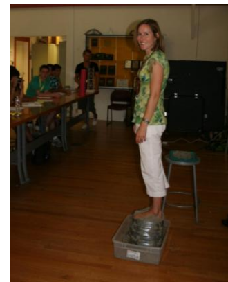
Figure 5: Sand with Duct Tape Confinement Supports Instructor's Weight
