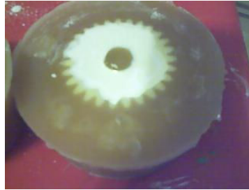
Figure 13: Plaster solidification in the mold.
