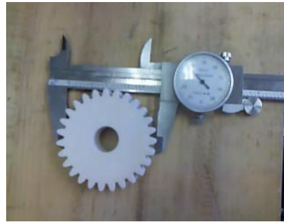
Figure 16: Measuring the components with profile comparator and Vernier caliper
